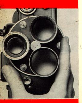
locking catch, thus freeing it (27). To swivel the turret (either clockwise or antichlockwise), use the three knobs fitted between the lenses, to avoid any risk of modifying their settings. Once the catch has clicked into place, the lens chosen for filming is properly aligned (upper position) (28).
