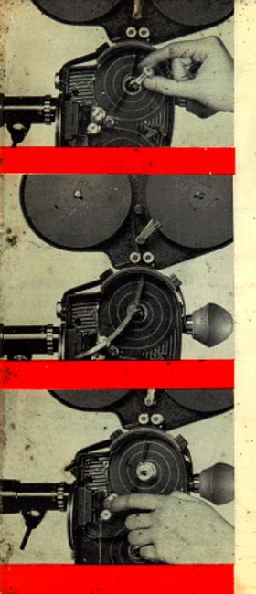
retaining screws should only be loosely tightened.
